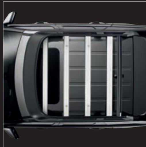
Expedition Roof Rack* CAB500130PMA For vehicles with Roof Rails, Fitting Kit (VUB504230) is required. Load capacity 54.3kg.
