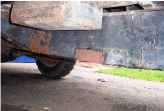
This patchwork quilt is even worse than it looks. The bottom face of the chassis was so rotten I could poke my fingers through it. The vehicle actually looked quite smart from above...
