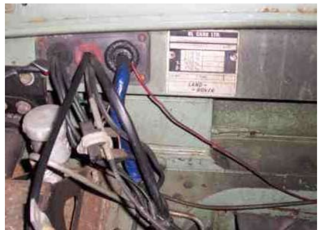
Chassis plate on later Series III (bonnet removed)
