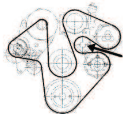
Discovery Series II ACE-equipped Belt Routing
