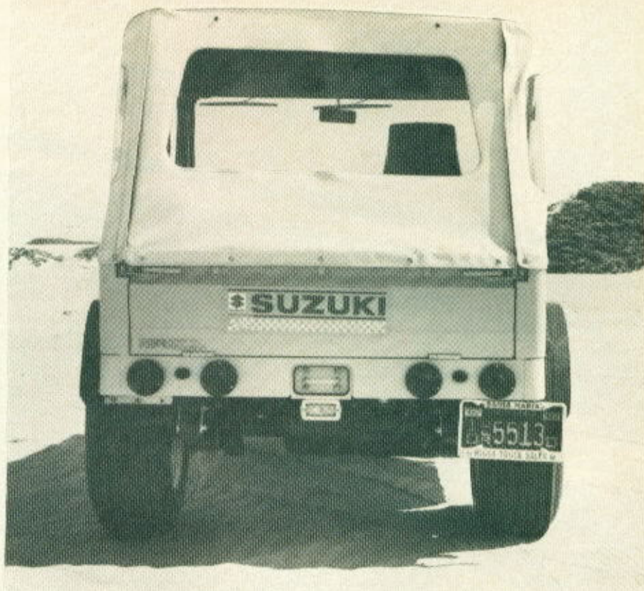
Overall height is 64.8 inches at the windshield and length is 117.9 inches. Total weight for the Suzuki Brute IV, unloaded, is 1350 pounds.
