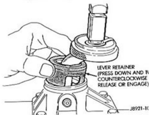
Fig. 3 Disengaging/Engaging Shift Lever Retainer
