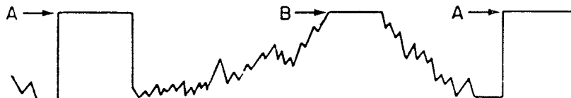
Figure 5 Overloaded or Clipped Video and Sync Signal.
