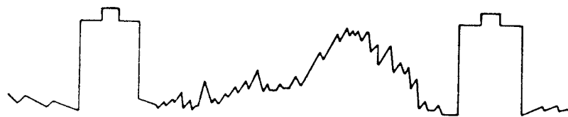
Figure 4 Normal Video and Sync Signal.
