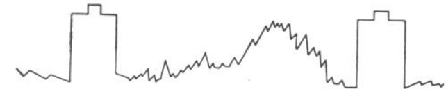
Figure 4 Normal Video and Sync Signal.
