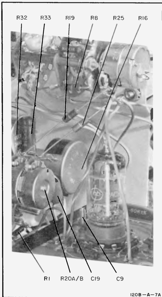
Figure 5-4. Right-Side View, Side Panel Removed, Location of Parts and Adjustments
