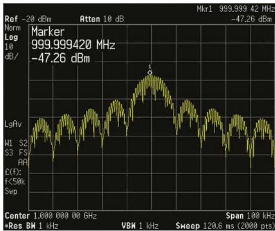
Figure 15. The bandwidth was changed to equal the pulse repetition frequency and the pulse width was changed to 0.1 ms.
