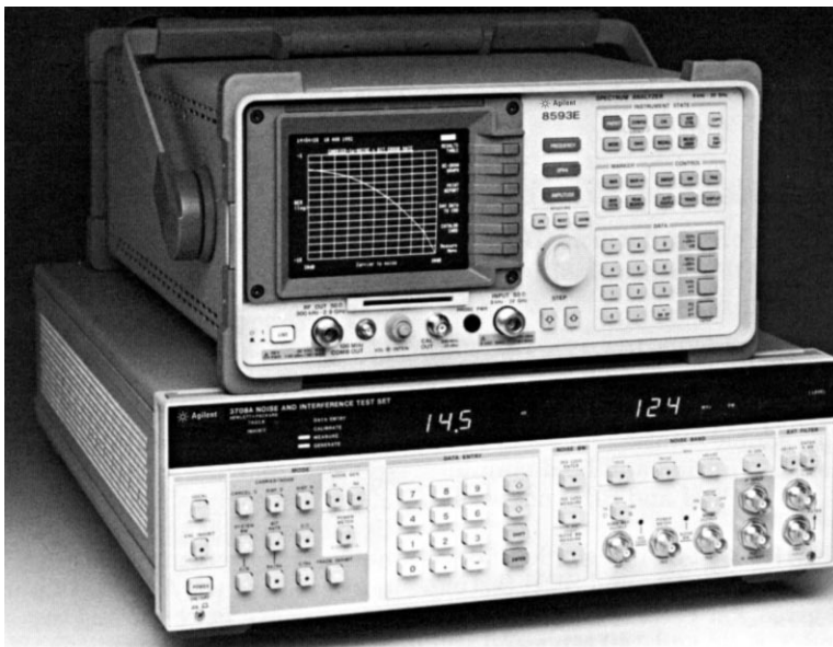
The C/N vs. BER Measurement Personality allows an Agilent 8590 Series spectrum analyzer to control the 3708A to make automatic measurements.
