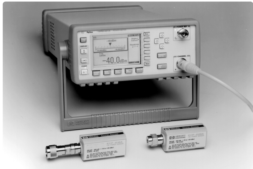
Figure 4-11. E4418B features many user-conveniences and a 90 dB dynamic measurement range. The 50 MHz, 1 mW reference output connector is at the top-right.
