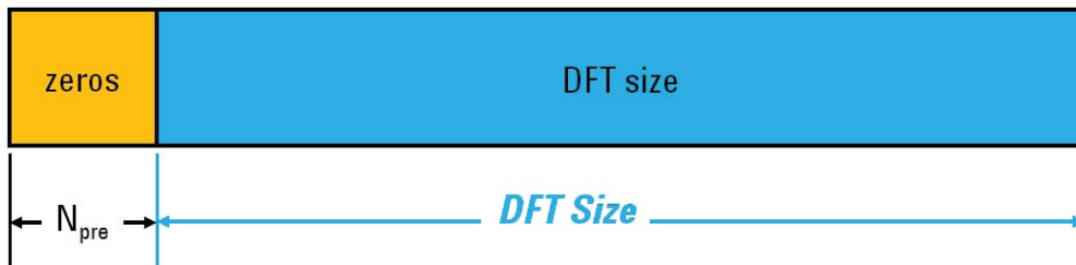
Figure 3(b) Payload OFDM symbol with zeros prefix
