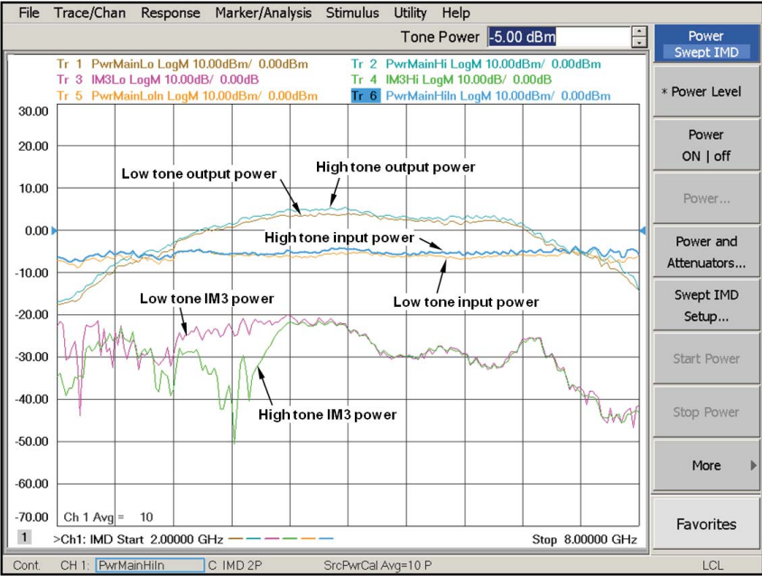
Figure 31a. Wideband pulse swept-frequency IMD measurements with open loop leveling
