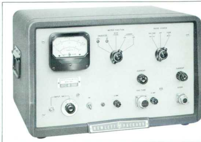
Fig. 2 (above). New Model 343A diode type VHF Noise Source provides flat noise output up to 600 megacycles without tuning for convenient testing of 50-ohm input receivers. Internal matching network compensates for transit-time effects in diode.
