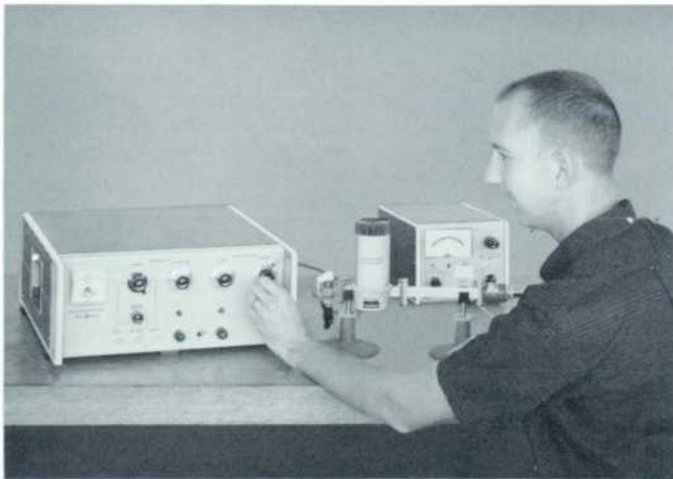
Fig. 1. New Klystron Power Supply permits high-performance operation of klystrons in exacting, present-day applications.
