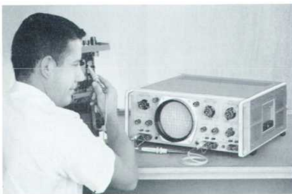
Fig. 1. New -hp- Model 130C Oscilloscope has a high sensitivity of 200 microvolts/cm and many conveniences to permit measurements to be made in presently-difficult situations. Scope uses new -hp- internal-graticule cathode-ray tube which avoids mirroring and parallax.
