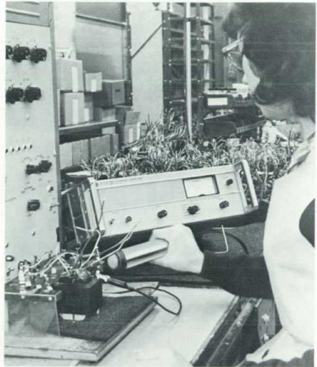
Ultrasonic inspection of high-voltage filament transformers for corona, using new Model 4950A Ultrasonic Translator. Translator alarm light indicates too much corona. Test voltage is 3.5 kV.
