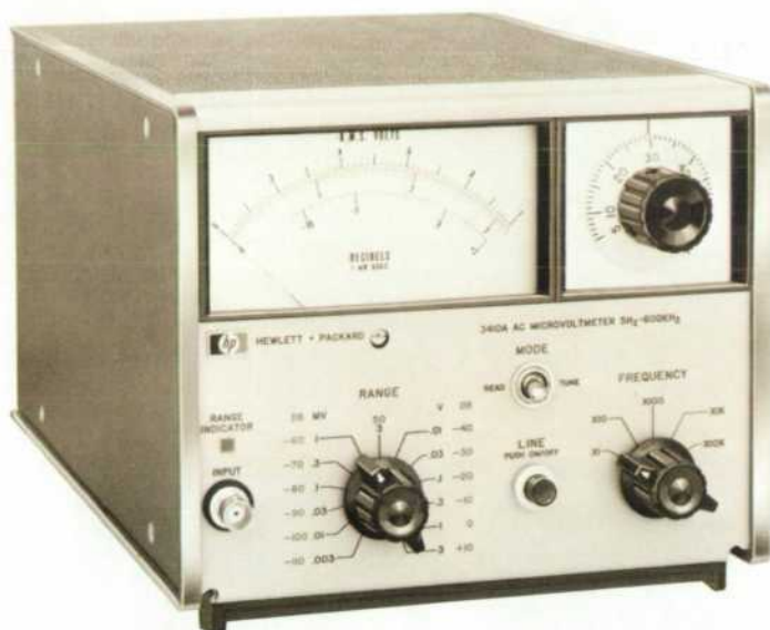
Fig. 1. This new all solid state -hp- Model 3410A AC Microvoltmeter will measure signals even when frequency and amplitude are unknown. A panel light helps in determining the proper setting of the range switch. Adjusting the front panel tuning control to within 1% of the signal frequency enables the phase-lock circuitry to lock on and track the input signal within the specified limits.
