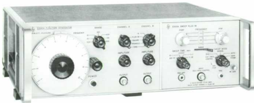
Fig. 1. Sweep frequencies from 0.1 Hz to 100 kHz, available from the Model 3305 Sweep Plug-In, permit quick and accurate testing of equipment ranging from subaudio through ultrasonic.
