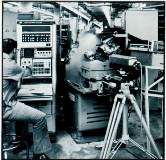
Fig. 2. New Model 5451A Fourier Analyzer, a minicomputer-based, keyboard controlled, dual-channel analyzer, can do spectrum analysis, correlation, coherence analysis and many other complex data manipulations. New capabilities are 80-dB dynamic range, relocatable software, buffered input, and a faster computer.
