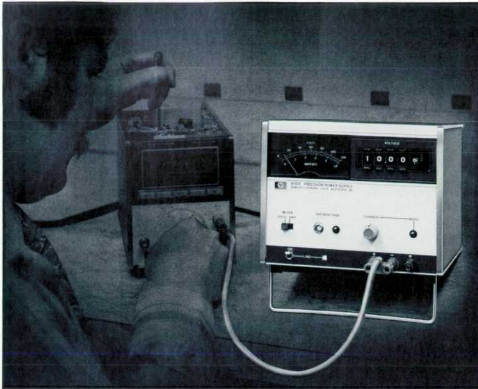
Fig. 1. Model 6115A Precision Power Supply has 4-digit push-button switch for quick setting of voltage. Vernier enables output voltage to be selected with 0.2 mV resolution. Output range is 0–50 V at 0.8 ampere, and up to 100 V at 0.4 A. Model 6114A is identical except for output voltage and current ratings (0–20 V at 2 A, up to 40 V at 1 A).
