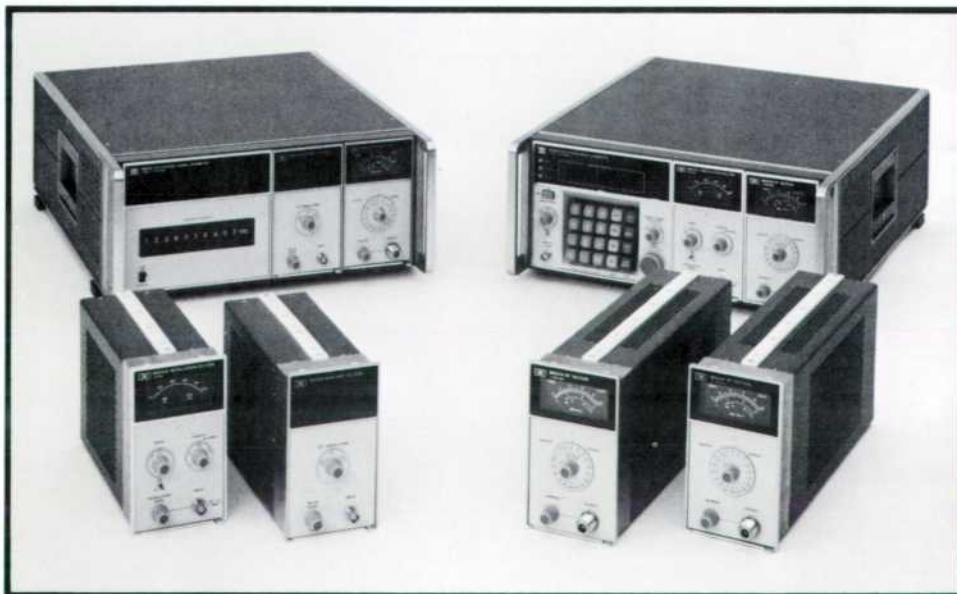
Fig. 1. Model 86602A 0.1–1.3 GHz RF Section (right foreground) is newest member of HP 8660-series Synthesized Signal Generator family. Other RF Section (Model 86601A) covers 0.01–110 MHz range. Family also includes two Auxiliary/Modulation sections (left foreground). Model 8660A mainframe (left rear) with switch selection of frequency is intended primarily for automatic test systems. Model 8660B (right rear) has pushbutton control of frequency that also gives automatically sequenced step-wise frequency sweeps. All functions operable from front-panel of all plug-in sections and both mainframes (frequency, output level, modulation, modulation depth) are programmable.
