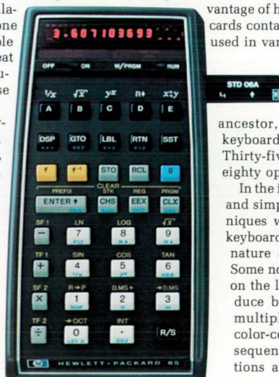
Fig. 1. The first fully programmable pocket calculator has 51 preprogrammed operations, a 100-step program memory, five user-definable keys, and a tiny magnetic card reader-recorder. After a program card is read it can be placed in the window above the keyboard to show the new functions of the user-definable keys.
