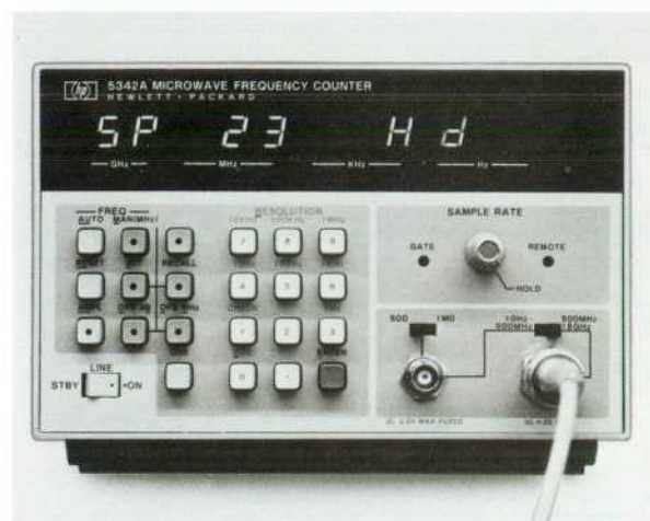
Fig. 1. Nine diagnostic modes are available with the counter in AUTO mode. The SET key is pushed twice and is followed by the appropriate digit key.
