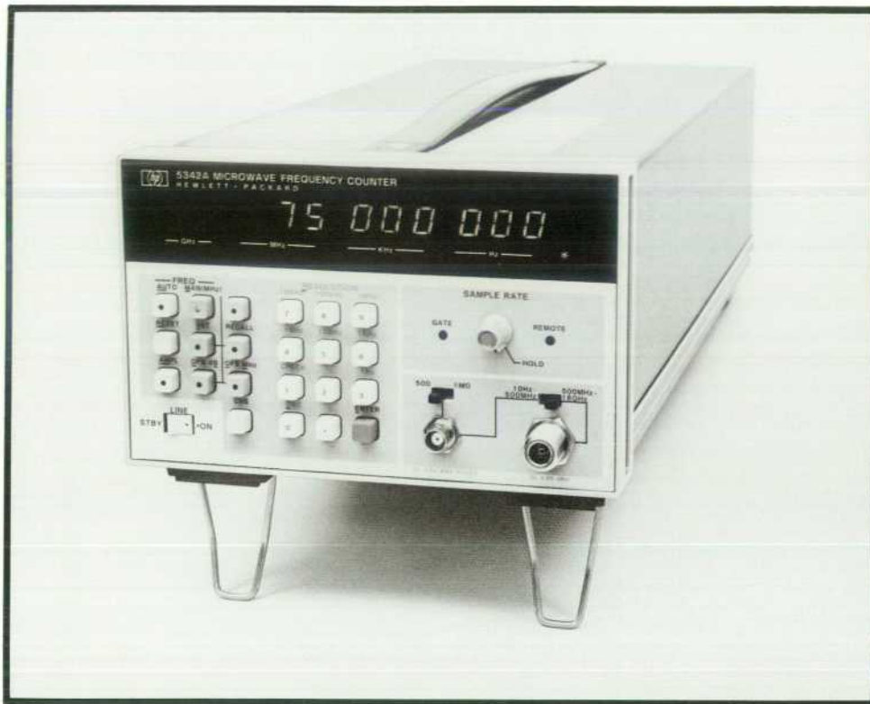
Fig. 1. Model 5342A Microwave Frequency Counter measures frequencies from 10 Hz to 18 GHz. With its amplitude measurement option, it can simultaneously measure and display frequency and amplitude. Keyboard control and microprocessor architecture provide ease of operation and data manipulation features.
