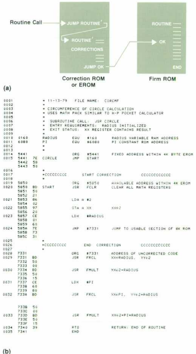
Fig. 2. (a) Relationship of the correction ROM to the firm ROM for a routine that has been corrected. (b) 6800 microcode example.
