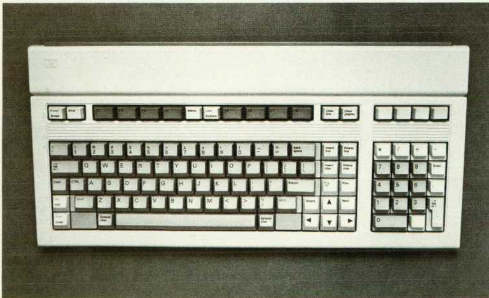
Fig. 1. The HP 46010 Keyboard is produced in seventeen local language versions for the HP 150 Personal Computer. Related keys are grouped together. Color is used to separate blocks (see Fig. 3).
