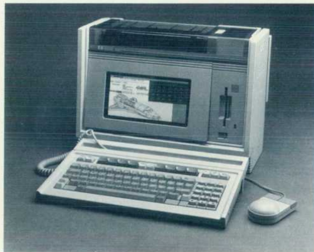
Fig. 2. HP's Integral Personal Computer 2 is a powerful multi-tasking computer system in a 25-lb transportable package. Designed for technical professionals, it features a built-in printer, display, disc drive, and HP-IB interface and the HP-UX operating system, HP's version of AT&T Bell Laboratories' UNIX ™ operating system.
