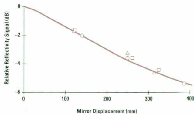
Fig. 6. The effect of dispersion mismatch on the peak interference signal from similar reflectors located at different locations with respect to the scan path of the movable mirror.
