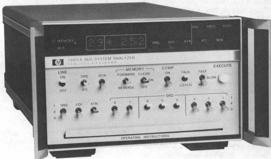
Figure 1. HP 59401A Bus System Analyzer is the technician's tool for bench testing the bus capabilities of a single instrument. The analyzer acts as a listener, talker, or controller for complete testing of an instrument.
