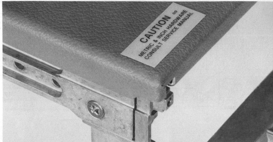
Yellow warning label on cover cautions that instrument uses mixed metric and inch fasteners.
