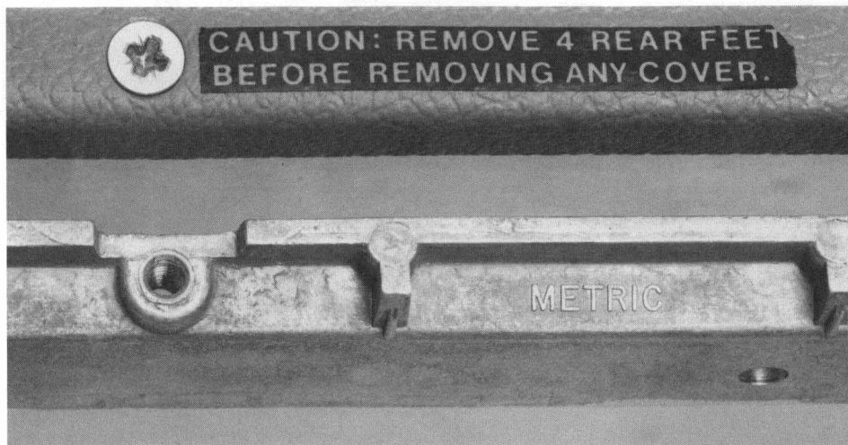
Rear bezel casting has metric mark alongside the top cover-attaching screw.
