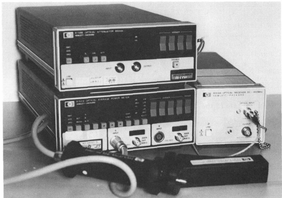
Figure 2. HP fiber-optic test equipment.
