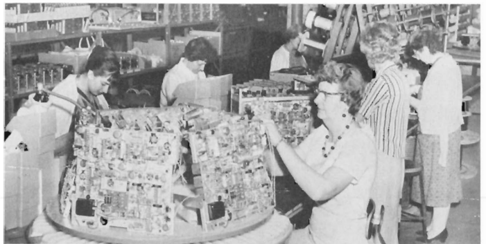
ABOVE: Modern production lines utilize "lazy Susans." Women here are assembling FM stereo modulators. BELOW: George Sanford demonstrates application of a BRC FM-AM signal generator with a Dymec servo programmer. System reduces tedious calibration to a push-button operation.
