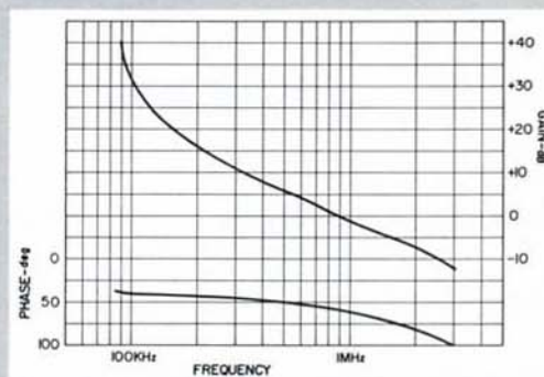
Figure 17: Operational amplifier high-frequency, open-loop gain/phase response.
