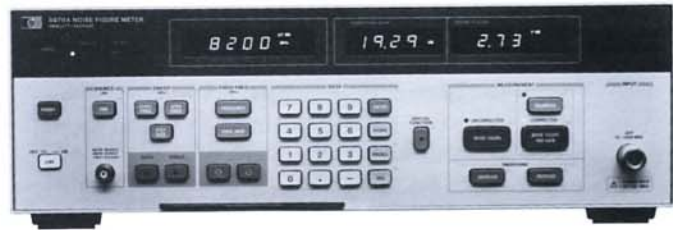
Figure 2-1. The HP 8970A Noise Figure Meter that includes a microprocessor to relieve the many operations involved in data collection and manual error correction that traditionally accompanied accurate noise figure measurements.
