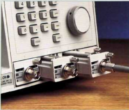
Input Pods for the HP 54100/54110 Oscilloscopes and the HP 54300A Probe Multiplexer.
