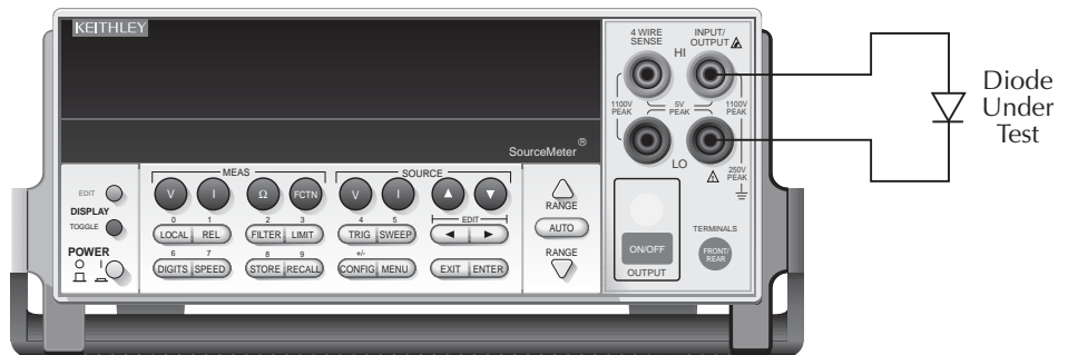
Figure 10-8 Connections for diode I-V tests
