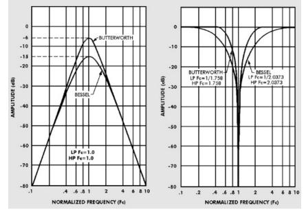
Set the filter to Butterworth response and apply 1Vrms at 10kHz to the INPUT of channel n.1 set to a low cutoff frequency of 1kHz. Set the filter to channel n.2 and the high cutoff frequency to 100kHz.
