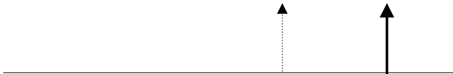
Figure 4. Interval Trigger that triggers when the interval width is smaller than the selected interval. The broken, upward-pointing arrow indicates a potential trigger, while the bold one shows where the actual trigger occurs — on the positive edge within the selected interval.
