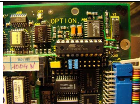
Slot A 8MB or Slot A and B 8MB (16MB total) Note: Both Jumpers are Horizontal
