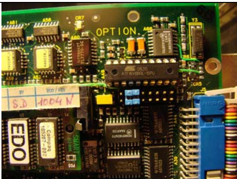
Slot A 4MB or Slot A and B 4MB SIMMS (8MB Total) Note: Both Jumpers are Vertical
