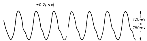
Fig. 4.12 Collector TR1 Schmitt trigger circuit
