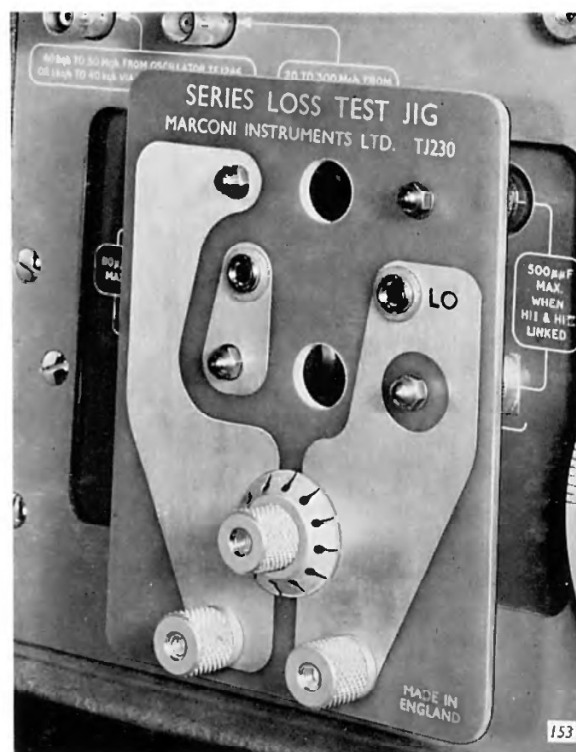
Fig. 2.2 Test Jig, Type TJ 230, fitted for Series Loss Measurements.
