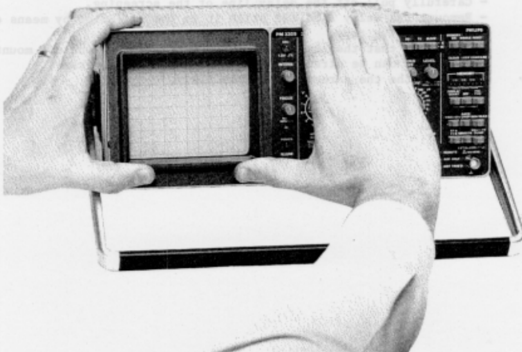
Fig. 7.10. Removing the bezel and the contrast plate
