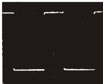
FIG. 12.8. Rounding due to incorrectly adjusted potentiometers
