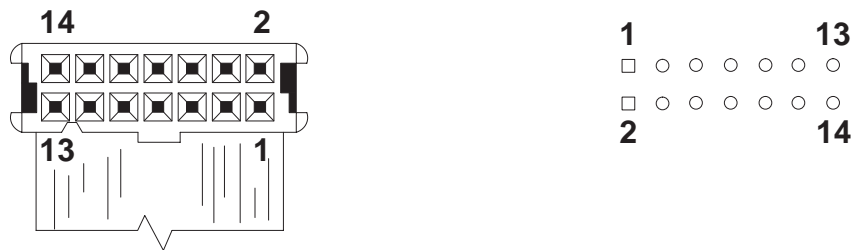
Connector plug P5040 on bottom of Main Board.
