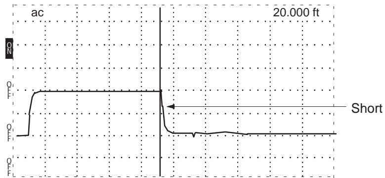
Figure 1-9: Short in the Cable
