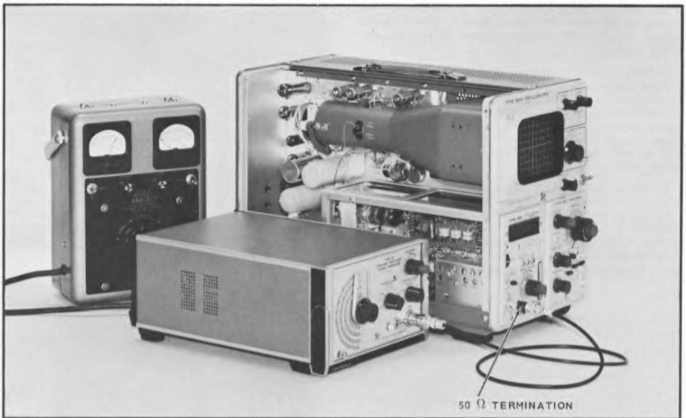
Fig. 6-22. Test setup for checking the Vertical Amplifier bandwidth, 10 mV/DIV.
