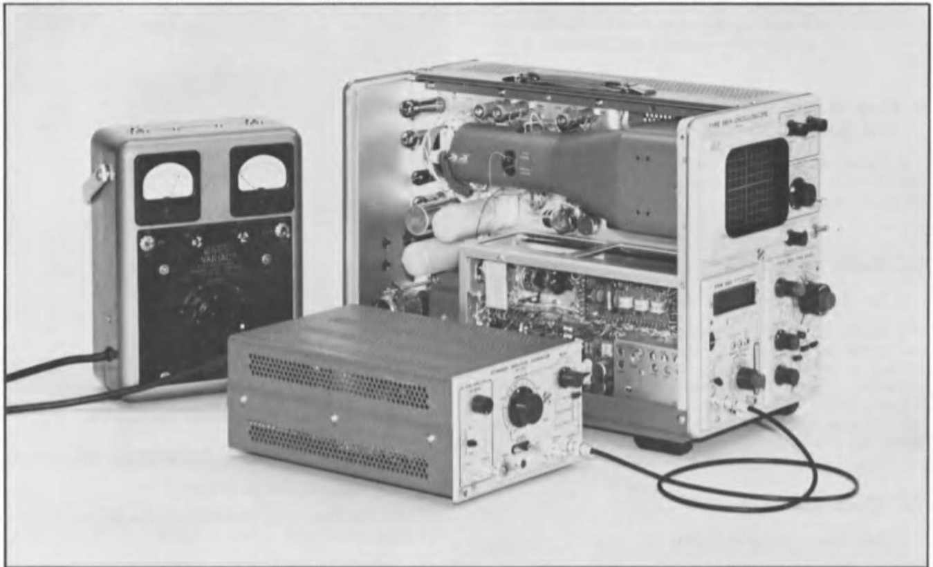
Fig. 6-7. Test setup for adjusting Vertical Amplifier gain.
