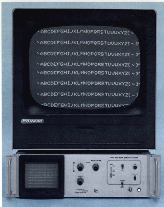
The information written on the 5-inch CRT of the scan converter (bottom) is converted to composite video and is displayed on the 17-inch CONRAC monitor (top).
