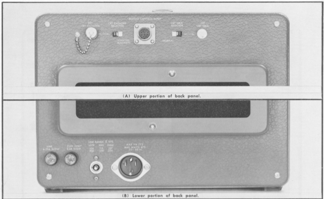
Fig. 2-2. Rear panel controls and connectors. (A) Upper portion of back panel. (B) Lower portion of back panel.
