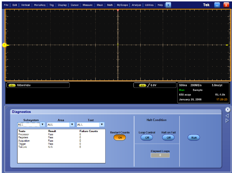
Figure 4-7: Diagnostics control panel
