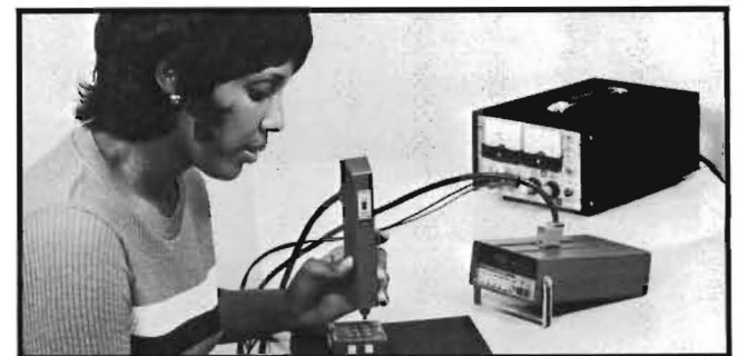
Fig. 6. The J6505 LED Test Probe being used for incoming inspection of light-emitting diodes by Brenda Bryant.
