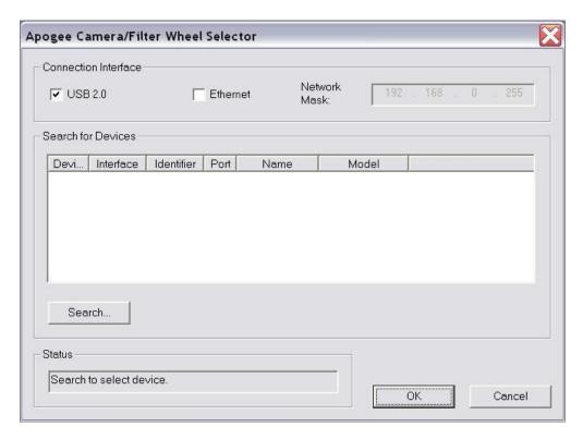
The **Apogee Alta Camera Selection Dialog** is displayed when the **Discover...** button is clicked. Select **USB 2.0** and/or **Ethernet**. If Ethernet, you must specify a **Network Mask**, which limits the subnet that is searched.
