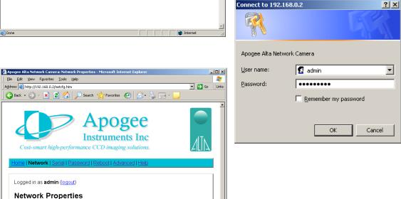
The **Network** page contains the TCP settings for the camera. From this page, the camera can be configured for a static IP network setup. Also on this page, the camera name can be selected (the
