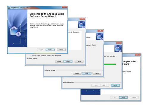
Upon successful driver installation connect your camera to the PC. Watch the message balloon in the lower right corner state the OS, search for and successfully install the drivers for the Apogee USB camera.
