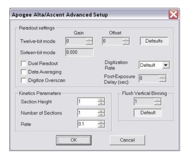
The **Gain** and **Offset** for Twelve-bit digitization mode can be changed from their factory values: you must unclick the **Defaults** button to unlock the edit boxes. The Gain for Sixteen-bit mode is not adjustable, but its value is displayed. You can also indicate whether to **Digitize Overscan** (the part of the CCD sensor surrounding the imaging area which is covered by an opaque mask). In some applications the overscan region is used as part of the calibration process.
