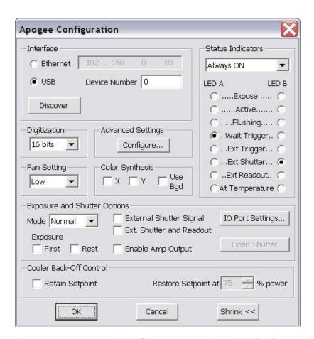
Alta cameras connected via USB can operate in two **Digitization** modes. The **12-bit** mode provides the highest speed, while the **16-bit** mode provides the highest dynamic range. Cameras connected via Ethernet support only **16-bit** mode.
