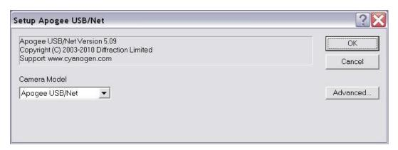
All settings for the Apogee camera are in the **Apogee Configuration** dialog, accessed from the **Advanced...** button. This dialog is also available while the camera is connected, by clicking the **Options** button on the **Settings** Tab and selecting the **Camera Settings** command.
