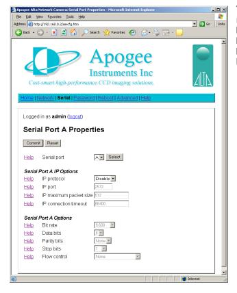
The **Serial** page lists all of the settings related to controlling the camera's onboard serial ports. The user can switch between Serial Port A and Serial Port B by changing the port from the drop down list.
