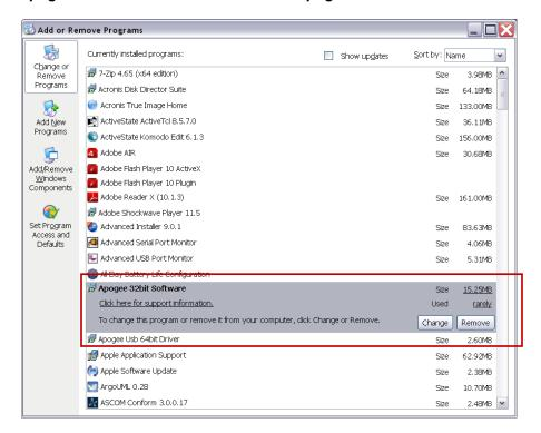
For Windows Vista/7 *Programs* dialog from the *Control Panel* and remove the *Apogee USB 64* or 32 bit Driver and the *Apogee 32bit Software*.
