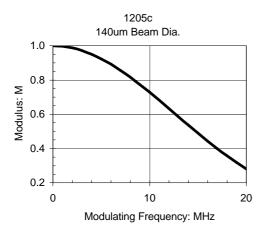
The typical MTF (depth of modulation) curve for the 1205C modulator assuming a 0.14mm beam diameter is shown at the left. For larger beam diameters the abscissa scales linearly. The curve is closely approximated by the function.
