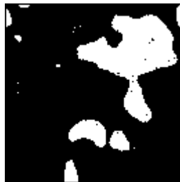
Figure 9-17. Binary Image before Application of Hit-Miss Function
